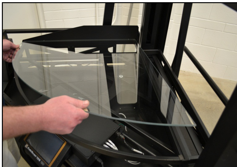
Figure 11 Glass Cubing and Weighing Platform
